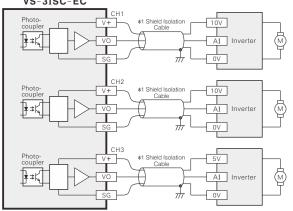
\*1: Please use the shield isolation cable and keep that away from power lines to minimize external interference. Besides, ground the shield of the signal cable (Class 3 grounding; earthing resistance < 100Ω)
